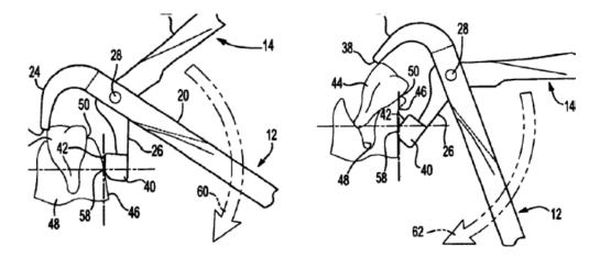
('890 patent Figs. 4, 5.) Using the method of claim 1, a dentist does not simply grasp the tooth with pliers and pull up on the tooth to remove it from the gum; instead, a dentist leverages the tooth from the gum by rotating the dental pliers around a fulcrum. The parties refer to the end of the dental pliers that grasps the tooth as the "beak" (labeled 24 in the pictures) and the end of the pliers that creates a pivot point as the "bumper" (labeled 40).
